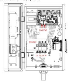
In clusters of chargers in a parking garage, a single EN-GATE can act as the communication gateway for maximum 12pcs chargers. Connect the EN-GATE with Charger #1 and the other chargers connect one by one with network cables between the CAN ports. The length of network cable between EN-GATE and Charger #1 should be  $\leq$ 10M. The total length of network cables from EN-GATE to the farthest charger should be  $\leq$ 100M.
